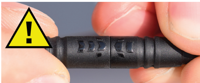
[Fig. 6] Carefully press plug together
